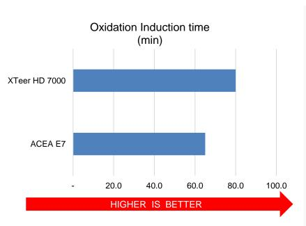
XTeer HD7000 meets the long oil drain requirements of Caterpillar, ACEA E7, API CI-4 from the Euro-5 to older generation engines, to allow operators to optimize maintenance schedules and control maintenance costs.
